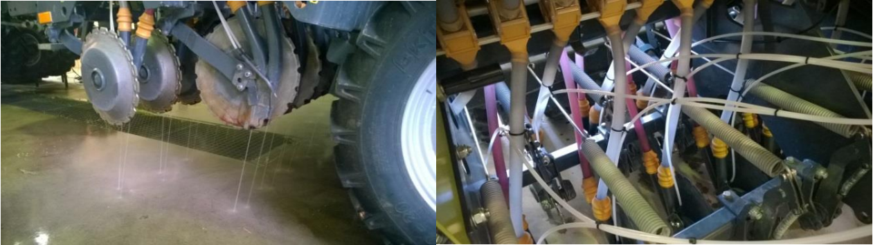
Fig. 6. Additional hoses for liquid fertilizers (thin white hoses) assembled to the combined seed drill (left). Special disc coulters, where liquid fertilizer hoses are attached to, enabling placement application of additional two liquid fertilisers (right).
