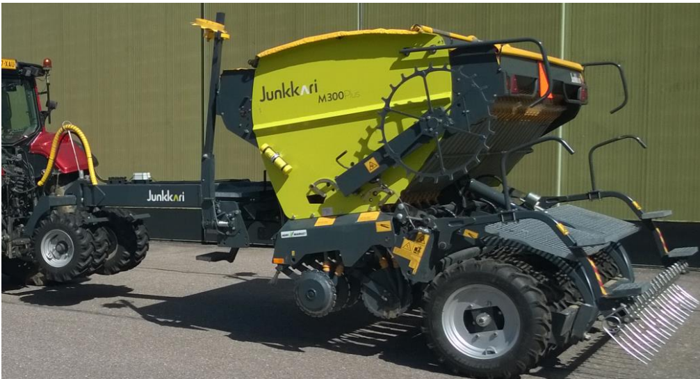
Fig. 5. Junkkari M300 Plus combined seed drill with four site-specifically controllable containers; 1 for cereal seed, 1 for granule fertilizer, 2 for small seeds (cover crops).
