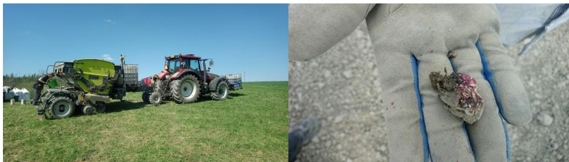
Fig. 11a and 11b. The machinery combination used in the field demonstration in a service break at Toivon Tila (left) and a typical soil-seed-fertilizer aggregate formed in the coulters and clogging them frequently (right).
