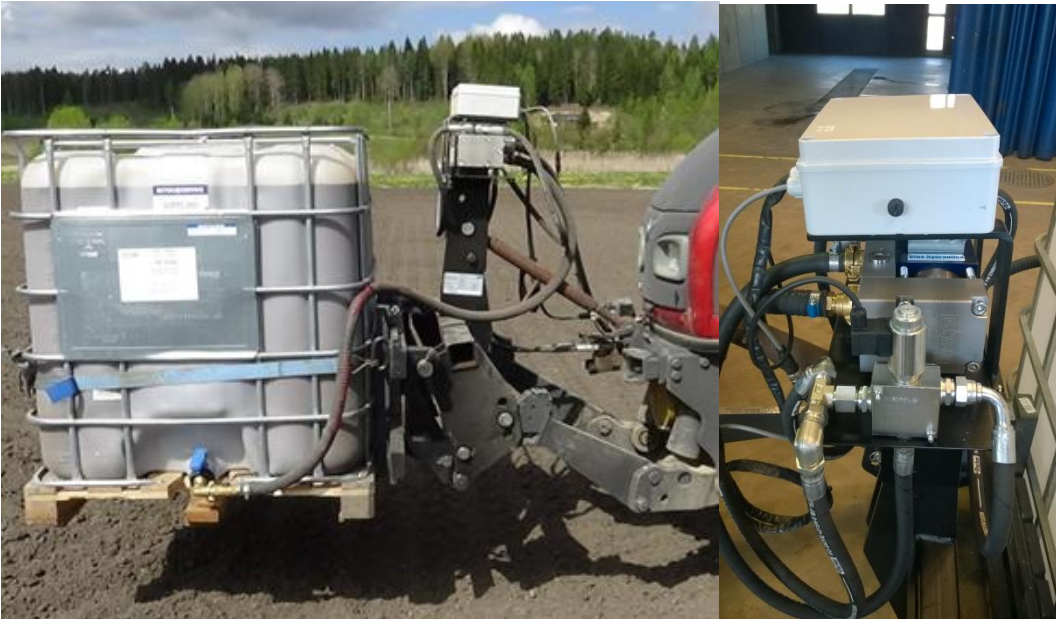
Fig. 7. Bio-Kali container in the front of the tractor (left) and the ISOBUS compatible controller (grey box) and liquid fertilizer pump for Bio-Kali application.
