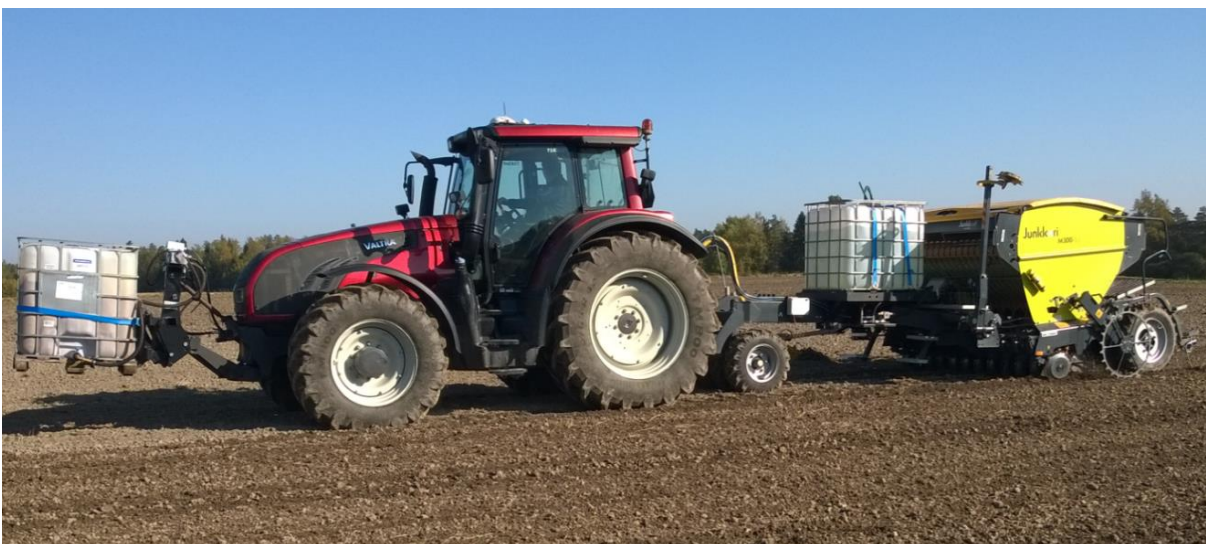
Fig. 9. The CIRCWASTE work set used in the field demonstration as a whole, enabling site-specific control of six independent inputs; seeds and fertilizers. Bio-Kali tank is located in the front of the tractor and AMS tank between the tractor and drilling machine.
