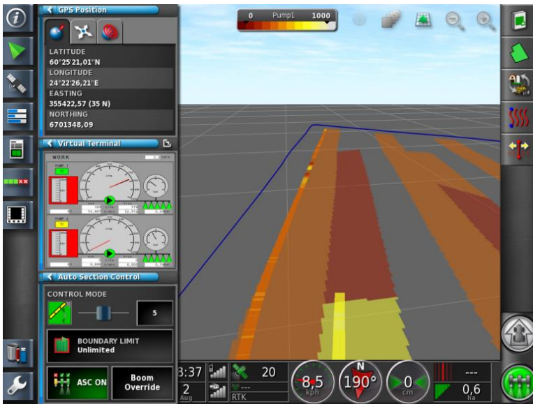
Fig. 8. ISOBUS compatible Valtra C3000 Task controller as a user interface for the machine combination.
